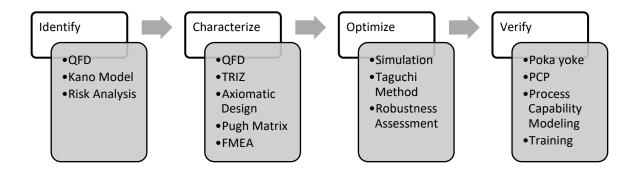
Figure 6 Phases and tools for engineering design process
